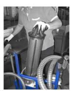
Unscrew the lower fastening nut, slide out the spacer and then the contaminated filter element.
