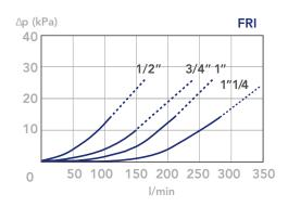
CLEAN FILTER ELEMENT PRESSURE DROP WITH F+, C+ AND M+ MEDIA (depending both on the internal diameter of the element and on the filter media)
