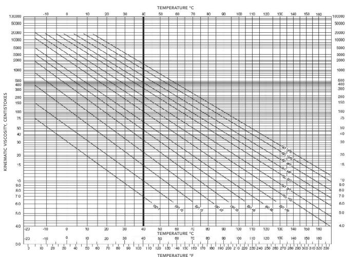
Lines shown refer to oils of ISO preferred grades and V.I. = 100. Lower V.I. oils will show steeper slopes. Higher V.I. oils will show flatter slopes. CENTISTOKES
