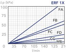
All the curves have been obtained with mineral oil having a kinematic viscosity 30 cSt and specific gravity 0,86 kg/dm3; for fluids with different features, please consider the factors described in the first part of this catalogue. All the curves
