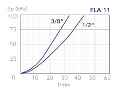
CLEAN FILTER ELEMENT PRESSURE DROP WITH M+ MEDIA (depending both on the internal diameter of the element and on the filter media)
