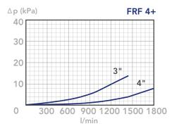
CLEAN FILTER ELEMENT PRESSURE DROP WITH F+, C+ AND ME MEDIA (depending both on the internal diameter of the element and on the filter media)
