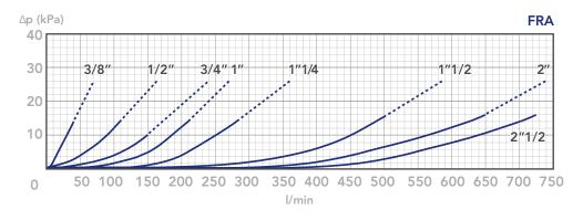
CLEAN FILTER ELEMENT PRESSURE DROP WITH F+, C+ AND ME MEDIA (depending both on the internal diameter of the element and on the filter media)
