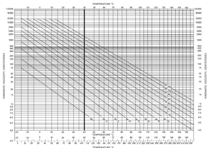
Lines shown refer to oils of ISO preferred grades and V.I. = 100. Lower V.I. oils will show steeper slopes. Higher V.I. oils will show flatter slopes.
