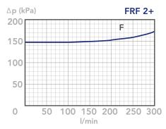
CLEAN FILTER ELEMENT PRESSURE DROP WITH F+, C+ AND ME MEDIA (depending both on the internal diameter of the element and on the filter media)
