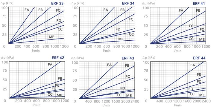
BYPASS VALVE PRESSURE DROP
