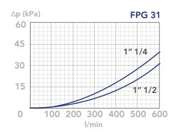
CLEAN FILTER ELEMENT PRESSURE DROP WITH F+ AND C+MEDIA (depending both on the internal diameter of the element and on the filter media)
