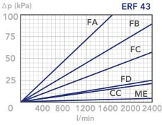
be lower than 50 kPa (0,5 bar) and should never exceed 1/3 of the bypass valve setting.
