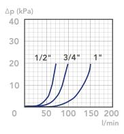
CLEAN FILTER ELEMENT PRESSURE DROP WITH F+ AND C+ MEDIA (depending both on the internal diameter of the element and on the filter media)
