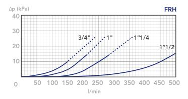
CLEAN FILTER ELEMENT PRESSURE DROP WITH F+, C+ AND ME MEDIA depending both on the internal diameter of the element and on the filter media)
