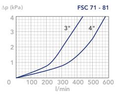
CLEAN FILTER ELEMENT PRESSURE DROP (pressure drop values of the elements by ME - MF - MG media are very similar)
