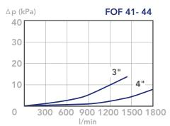
CLEAN FILTER ELEMENT PRESSURE DROP WITH F+, CC AND ME MEDIA (depending both on the internal diameter of the element and on the filter media)  $\frac{1}{2}$
