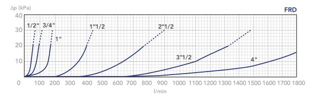
CLEAN FILTER ELEMENT PRESSURE DROP WITH F+, C+ AND M+ MEDIA (depending both on the internal diameter of the element and on the filter media
