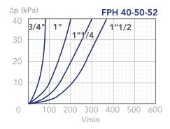
CLEAN FILTER ELEMENT PRESSURE DROP WITH F+ AND M+ MEDIA (depending both on the internal diameter of the element and on the filter media)
