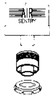
Adapter A-104 bayonet for standard flange
